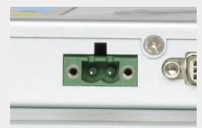
Phoenix terminal using fastening type power connector
