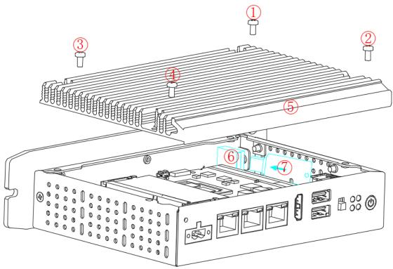
Figure 13 USB dongle Setup
