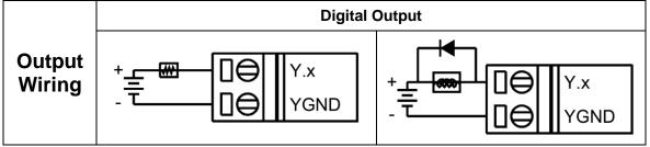
Figure 15 DO electrical wiring diagram
