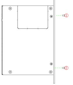
Figure 9 Attach the wall-mount part
