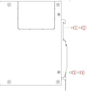
Figure 10 Attach DIN-Rail mounted part
